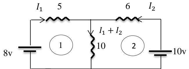
**EX.1:** For the circuit shown below calculate currents  $I_1, I_2, I_3$  using Kirchhoff's laws.
