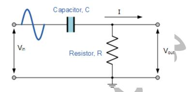
In this circuit arrangement, the reactance of the capacitor is very high at low frequencies so the capacitor acts like an open circuit and blocks any input signals at VIN until the cut-off frequency point (fC) is reached. Above this cut-off frequency point the reactance of the capacitor has reduced sufficiently as to now act more like a short circuit allowing all of the .input signal to pass directly to the output as shown below in the filters response curve
